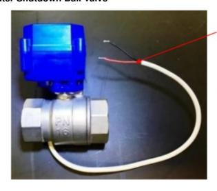
The 230VAC supply to the valves is generated from within the alarm unit. 15 to 25mm valves are supplied with a red and black cable, whilst larger valves are red and green. For good practice connect live to the red wire and neutral to the black or green wire. **WARNING:** In order to shut properly, this type of valve need powering for at least 3 minutes.
