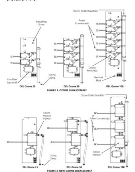
Restore power to the unit and check proper operation, including that the ozone module light(s) are illuminated. Close unit door.
