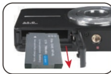
4.If you want to remove the battery please push the battery lock lever and remove the battery.
