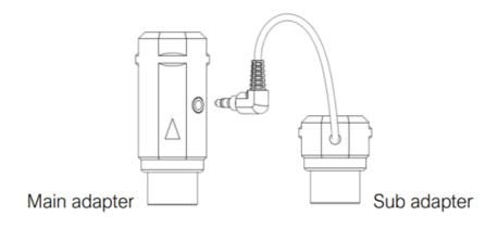
There is a push switch on the main adapter of WIDI Master, it is used for the following quick operations (please confirm that the product firmware has been upgraded to the latest version). The following operations are based on
