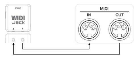
**Note 1:** The above picture shows the connection of the 5-pin DIN MIDI socket, and the connection method for other MIDI socket specifications is similar.
