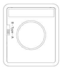
The slide switch on the back of the WIDI Jack can be used to switch the input / output polarity of the mini TRS jack to adapt to the two different TRS to 5-pin DIN MIDI cable specifications. Namely Type-A or Type-B (the optional TRS to 5-pin DIN cable from CME is TypeB). With this switch feature WIDI Jack can be applied to most TRS MIDI specifications in the market.
