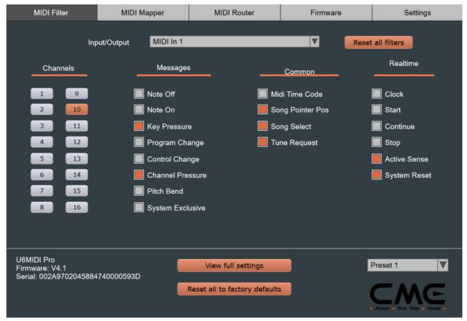
• [Reset all filters]: This button resets the filter settings for all ports to the initial state, in which no filter is active on any channel.
