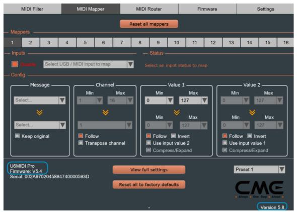
• [Reset all mappers]: This button clears all setting parameters from the MIDI Mapper page and the mapper in the connected and selected CME USB MIDI device, allowing you to start a new configuration of your MIDI Mapper settings.
