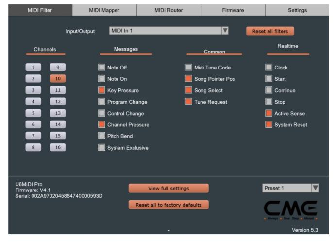
• [Reset all filters]: This button resets the filter settings for all ports to the initial state, in which no filter is active on any channel.
