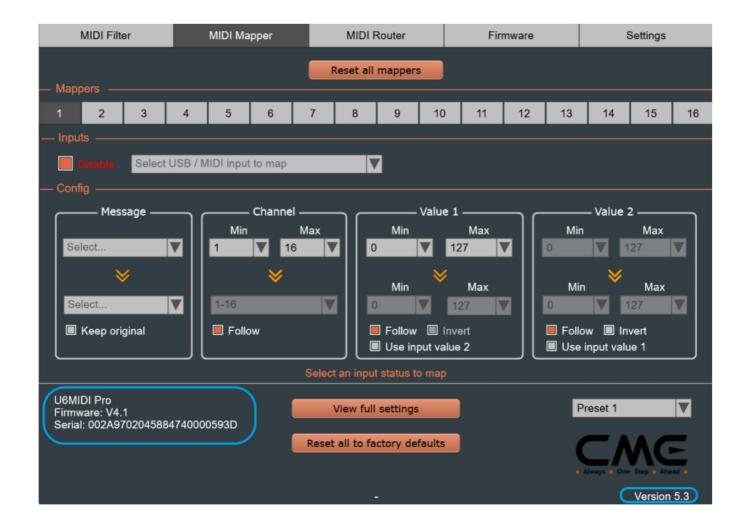
[Reset all mappers]: This button clears all setting parameters from the MIDI Mapper page and from the connected and selected CME USB MIDI device, allowing you to start a new configuration of your MIDI Mapper settings.
