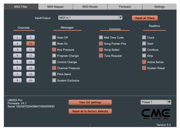
• [Reset all filters]: This button resets the filter settings for all ports to the initial state, in which no filter is active on
