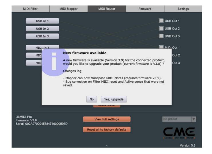
When the software cannot be updated automatically, you can manually update it on this firmware page. Please go to <a href="www.cme-pro.com/support/">www.cme-pro.com/support/</a> webpage and contact CME Technical Support for the latest firmware files. Select [Manual update] in the software, click the [Load firmware] button to select the downloaded firmware file on the computer, and then click [Start upgrade] to start the update
