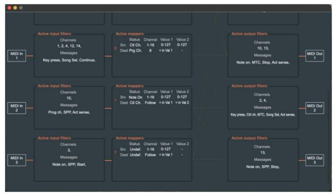
• [Reset all to factory defaults]: This button restores all settings of the connected and selected device by the software (including [Filters], [Mappers], [Router]) to the original factory default.
