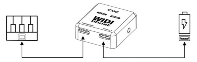
Plug the USB-B or micro-B connector of optional OTG cable into USB socket of the USB MIDI device, and then plug the USB-C connector into USB Host/Device socket on the left side of the WIDI Uhost.
