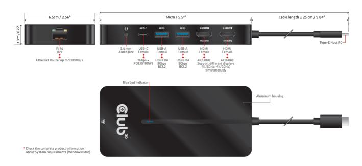
The Club 3D CSV-1595 USB Gen1 Type-C 7-in-1 hub with with 2x HDMI™, 2x USB Gen1 Type-A, 1x RJ45, 1x 3.5mm Audio, 1x USB Gen1 Type-C 100W Female port, provides a very advanced, efficient solution to extend a single USB Gen1 Type-C port to multiple ports.
