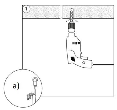
a) 5 core combi cable fitted with intergrated safety cable
