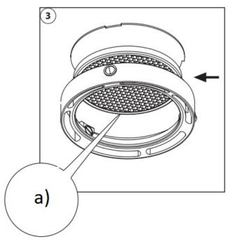
a) Make sure the honeycomb is placed between the diffuser & frontring
