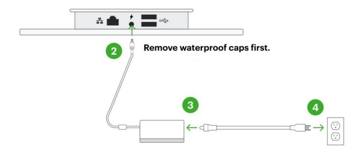
Plug in last, to a grounded AC power outlet.
