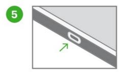
On PoE-enabled networks, the Power Over Ethernet port (IEEE 802.3at, PoE+) can be used as an alternative source of power.
