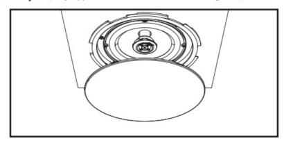
To attach the grill to the speaker, insert the lips into the provided openings on the speaker baffle and rotate it a partial turn (15°) to lock it into place.
