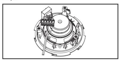
Strip the ends of the wires coming from the amplifier and insert in the spring-loaded terminal block connector on the loudspeaker. No screwdriver is required.
