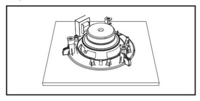
Fix the speaker in the provided opening by tightening the screws of the mounting clamps using a screwdriver. A quarter turn will cause the mounting clamps to flip-out, locking the speaker in place. Tighten the screws further until the speaker unit is fully secure.
