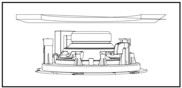
Make sure the mounting clamps are fully bent inwards, allowing the speaker fit through the cut-out. Insert the speaker to the opening.
