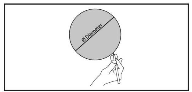
Cut a hole at the mounting location in the ceiling using the template supplied. You can check that the diameter is correct for the model by referring to the table above.
