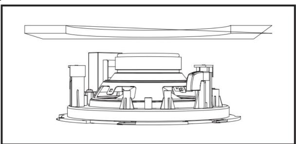
Make sure the mounting clamps are fully bent inwards, allowing the speaker fit through the cut-out. Insert the speaker to the opening.
