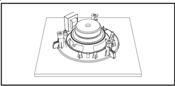
Fix the speaker in the provided opening by tightening the screws of the mounting clamps using a screwdriver. A quarter turn will cause the mounting clamps to flip-out, locking the speaker in place.
