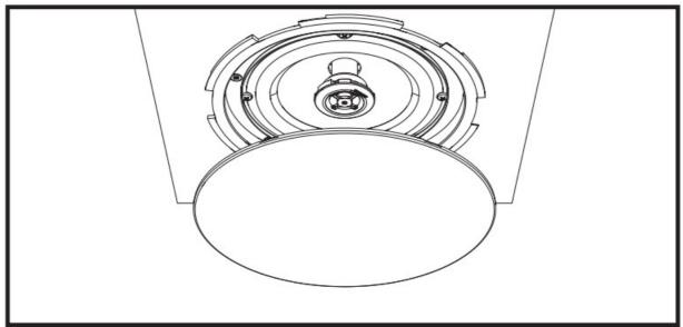
To attach the grill to the speaker, insert the lips into the provided openings on the speaker baffle and rotate it a partial turn (15°) to lock it into place.
