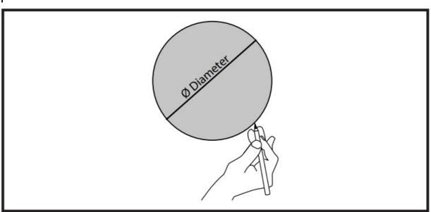
Cut a hole at the mounting location in the ceiling using the template supplied. You can check that the diameter is correct for the model by referring to the table above.
