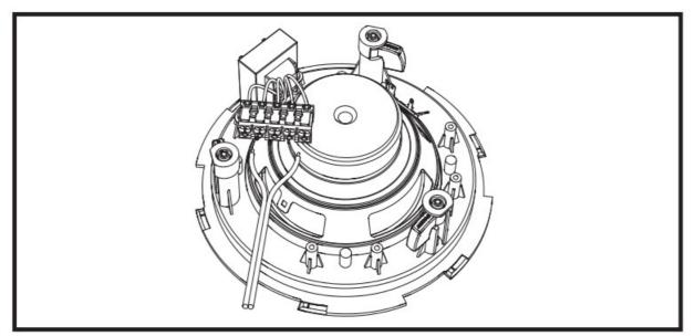
Strip the ends of the wires coming from the amplifier and insert in the spring-loaded terminal block connector on the loudspeaker. No screwdriver is required.
