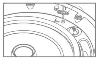
Place the bridge on back of ceiling tile. Align holes and insert speaker in hole. Tighten dog ears. Do not overtighten. (Tile bridge not available for C4.)
