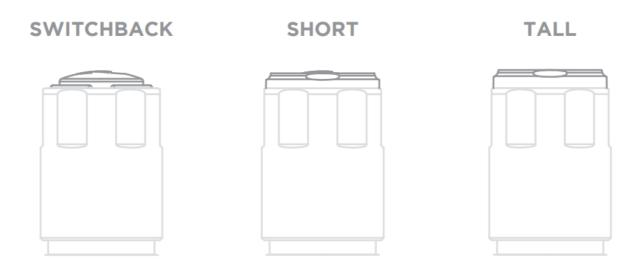
The MCH utilizes an industry-first feature that prevents accidental or negligent discharge of the light. Each MCH ships with 3 different ND Protectors that simply thread into the tail cap. They are replaceable at any time, should you want to adjust things.
