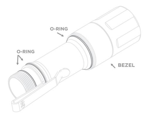
The o-rings on either side of the body: like all o-rings, can and will eventually fail. To prolong their life, periodically apply a small amount of non-petroleum based lubricant. Replacement o-rings can be purchased through www.clouddefensive.com
