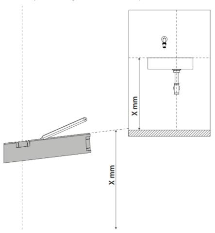
3. Mark with pencil the spots to drill holes. It is recommended to verify the given dimensions.
