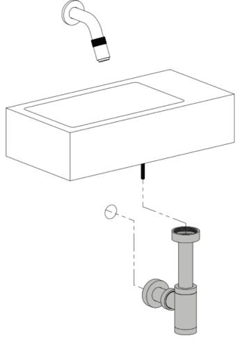
10. Adjust the height of the drain cap in a way that the water runs of fast enough.
