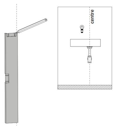
2. Mark with pencil and level the preferred height X of the hindbrain. (recommended: X = 900 mm)
