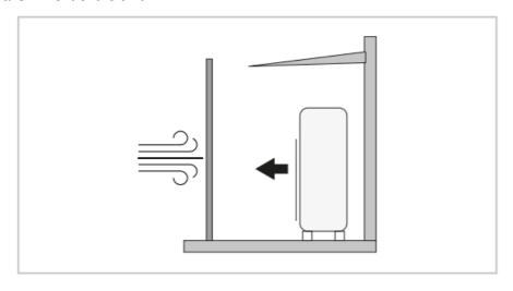
• Do not install the unit in a location where the suction side may be directly exposed to wind.
