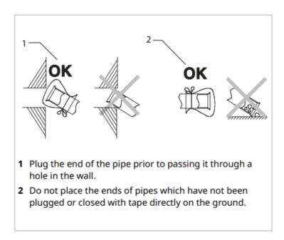
• If installation of the piping is not completed by the next day or for a long period of time, braze the ends of the pipes and fill with anhydrous nitrogen through a Schra-der valve access fitting to prevent moisture and particle contamination.
