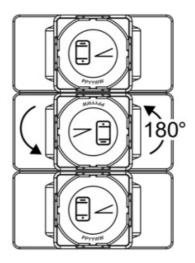
When installing in a 3-gang plate, the middle module must face the opposite way to the other 2 modules. The maximum load rating of each module must be derated (see Derating section).
