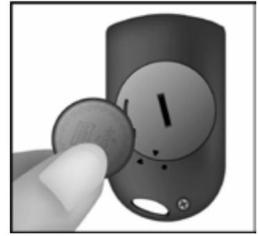
Step 1. Remove the battery cover by using a coin to turn it counter-clockwise.
