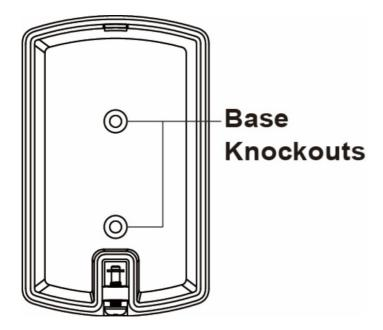
The base has two screw knockouts, where the plastic is thinner for mounting purposes. To mount the Panic Button:
