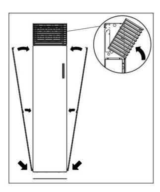
6. Place the side panel back on the device, then place the upper grille back. Press any button to leave the service mode.
