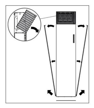
3. First remove the top grille of the device, then remove one of the side panels.
