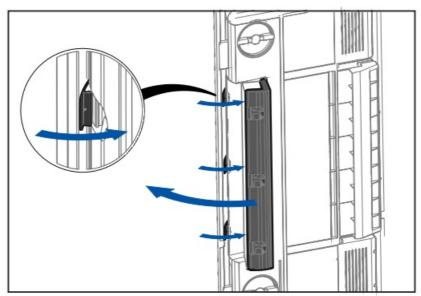
6. Cleaning the air outlet. When the filters do not yet have to be replaced, you can use a vacuum cleaner to clean the filters. You do not need to open the filter housing.
