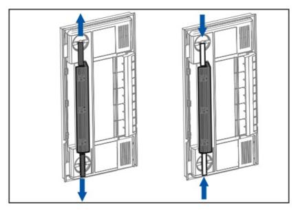
5. Close the filter housing and secure with the three clips. Caution: The filters must not protrude out of the filter housing.
