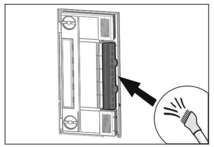
7. Replacing the air outlet filters. Unlock the filter housing by gently pulling the two clips towards you. Turn the filter grille as far forward as possible. Push the filters from the front out of the filter housing.
