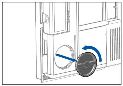
10. Remove the round cups from the air duct and remove the dust and dirt from the insect mesh.
