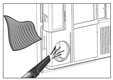
12. Insert the round cups.. Install both inspection hatches and tighten them well for a correct operation.
