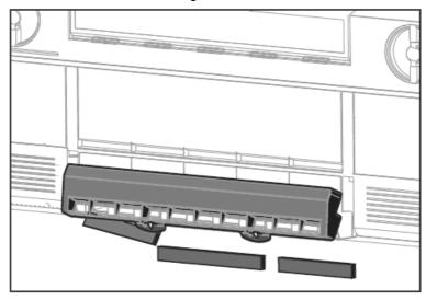
10. Press the grille at the bottom with the two clips firmly closed until you feel it snap. Please note that the filter housing must be properly closed for proper operation.
