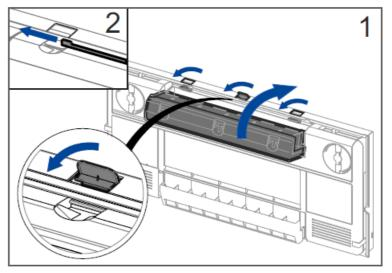
7. Cleaning the air outlet filters. When the air outlet filters are only slightly dirty, cleaning them with a vacuum cleaner is sufficient and you do not need to remove the air outlet filter.
