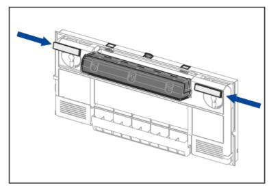
6. Close the filter housing and secure with the three clips. Caution: The filters must not protrude out of the filter housing.
