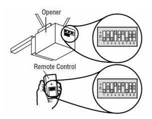
**TYPE 2**Genie, Linear and Moore-O-Matic garage door openers or receivers with 2 position DIP switches.
