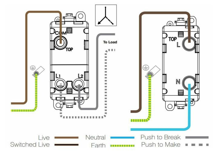
After making the connections, screw the switch plate accessory gently to the back box ensuring no wires become trapped.
