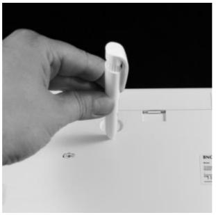
3. Press the Bluetooth pairing button on the backside of the Clevy Keyboard. The left blue led light (on the front of the Clevy Keyboard) is now blinking.
