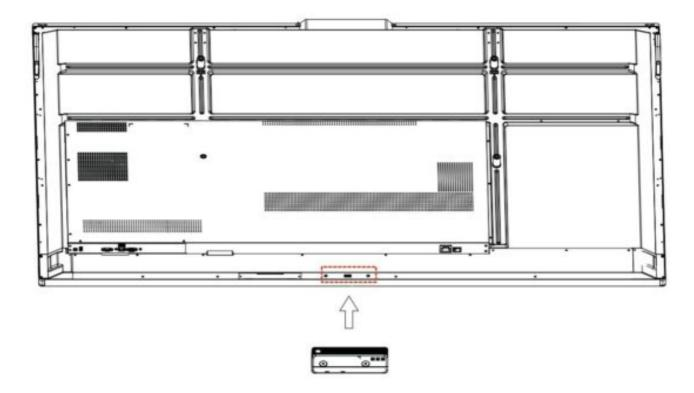
1) Position the Sensor Box to the bottom of the IFP in the direction of the arrow.
