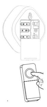
To pair multiple chimes to the same button, repeat the steps above. To pair multiple buttons to the same chime, remove the batteries from the chime each time you pair a new button. If the chime does not emit a sound during stage 2, press any button on the chime when the batteries are disconnected to remove any residual battery power, wait a short moment, and attempt to pair again.
