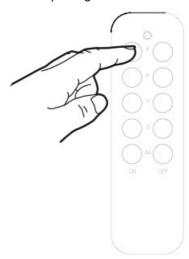
Repeat the steps for each plug you want to control. You can pair multiple plugs to the same channel. For example, to control all plugs in the living room using On/off on channel "A".
