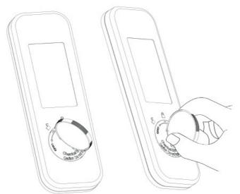
To replace a depleted battery, open the battery compartment and insert 1x CR2032 battery, mind the polarity.
