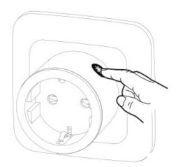
Note! If the indicator light starts flashing rapidly when you attempt to activate pairing mode, the button was held downfor longer 6 seconds and the receiver has entered reset mode (see "Resetting"). Make sure to release the button after 3 seconds.
