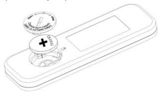
**Note!** It's important that the new battery does not touch the top of the battery compartment during installation as this can short circuit the remote control.
