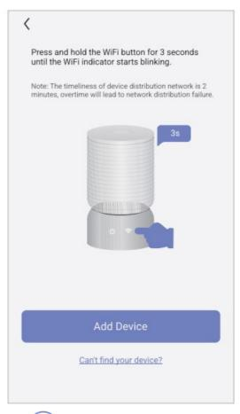
3. Select Wi-Fi ( ), enter your Wi-Fi ( ) password, and check the box "my Wi-Fi does require a password" then click connect. It will initiate the networking and Wi-Fi connection will be established.
