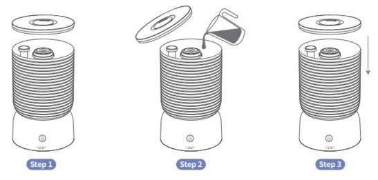
b. Removing the top cap and taking the water tank off of the unit base and then filling the water tank with water before returning it to the base.
