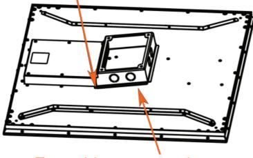
To avoid tape engaging prematurely, keep conduit box tilted until properly positioned.
