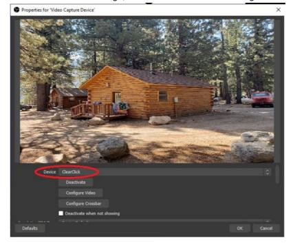
**NOTE:** If you wish to record at 4K resolution & 60 FPS, scroll down to the "Resolution/FPS Type" setting and choose "Custom." Type in "3840×2160" into the "Resolution" field. Select "60" under the "FPS" field.
