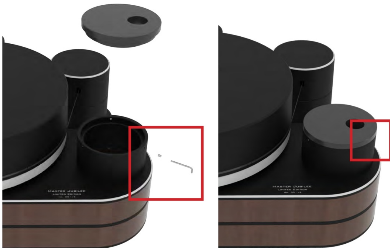
Pic. 5: Rough alignment of the tonearm base
