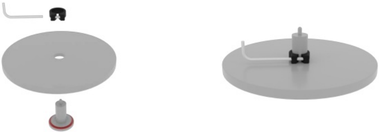
Pic. 7: Connection of sub-platter and bearing
