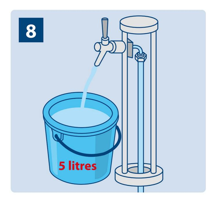
**FINAL FLUSH:** To ensure no traces remain in the system draw a further 5 litres of clean water then reconnect beer dispensing line.
