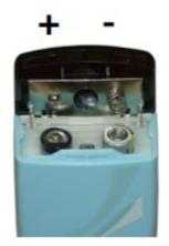
2. Install 2 AAA batteries. Make sure the + and – symbols on the metal hinge of the battery compartment correspond with the + and – end of each battery.
