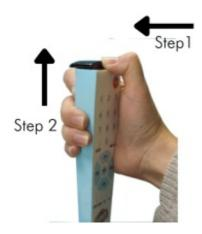
1. Looking at the keypad, slide the dark lens cover away from you (STEP 1) and lift the lid from the back (STEP 2).
