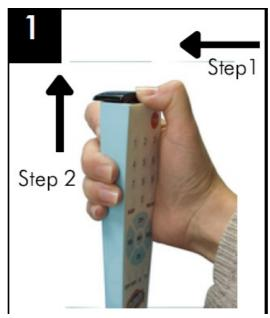
2. Install 2 AAA batteries. Make sure the + and – symbols on the metal hinge of the battery compartment correspond with the + and – end of each battery.
