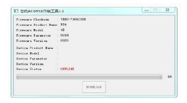
2. When the Dragon Shock 4 is in standby mode, long-press the SHARE and Cross buttons and connect the gamepad to the computer with the micro-USB cable provided. The controller driver will enter in update mode. Then select DOWNLOAD to launch the update. Refer to the second image below to see if the update was successful.
