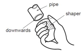
• Remove the burrs with shaper and prevent the burrs from getting into the pipe.
