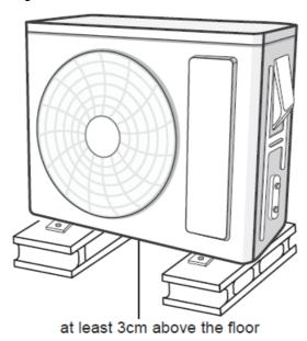
2. Fix the support of outdoor unit on the selected location with expansion screws.
