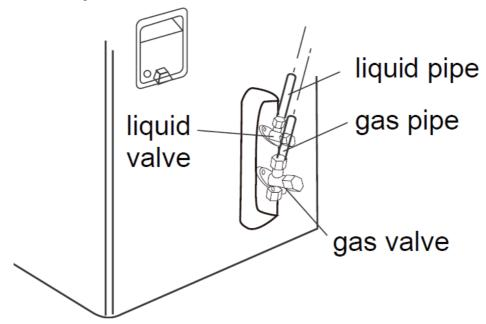
2. Remove the screw cap of valve and aim the pipe joint at the bellmouth of pipe.
