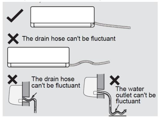
• Slant the drain hose slightly downwards. The drain hose can't be curved, raised and fluctuant, etc.
