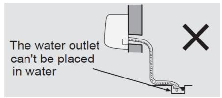
• The water outlet can't be placed in water in order to drain smoothly.
