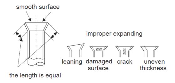
Check the quality of expanding port. If there is any blemish, expand the port again according to the steps above.
