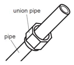
• Remove the union nut on the indoor connection pipe and outdoor valve; install the union nut on the pipe.
