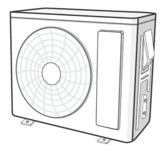
1. Remove the screw on the right handle of outdoor unit and then remove the handle.
