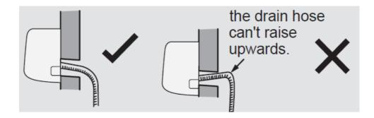
• The through-wall height of drain hose should not be higher than the outlet pipe hole of the door unit.
