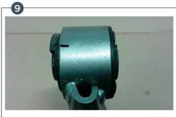
△ **ATTENTION**: Apply grease to screw around nut rotation area, and also oil silentblock seat before insertion.
