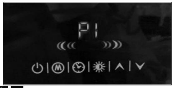
4. Press to select the mode from P1-P6, referring to the different temperature settings.
