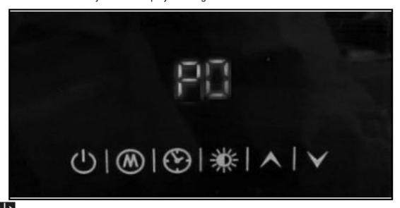
3. Press to turn on the upper heating lamp and the screen will show P1.
