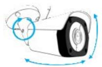
11. Adjust the camera by panning, tilting, and rotating the camera body to the desired viewing angle.
