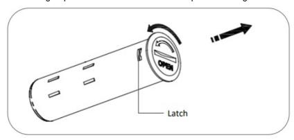
2. Pulling out the hardware from the plastic casing to change the battery.
