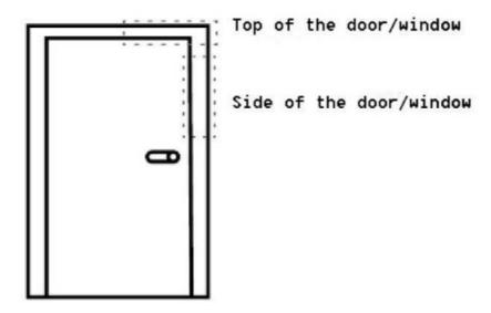
The rectangular areas highlighted above are optimal installation positions.
