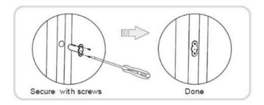
With your door/window and door/window frame prepared and the drill holes created, it's now time to mount both parts of your Recessed Door/Window Sensor.
