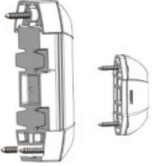
3. Mount the magnet into the desired location making sure the magnet alignment mark lines up with the sensor mark.
