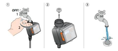
At the end of the season, before the winter frosts, disconnect the timer from the tap, remove the batteries and store it in a closed environment, away from damp, where the temperature does not fall below 3°C.
