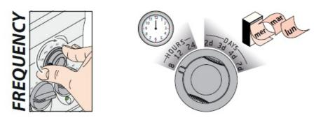
**PROGRAMMING – Immediate irrigation start.** To start the program immediately, press START+...once. The next watering cycle will begin after the time period set with the FREQUENCY selector has elapsed. Timer scheduling is based on when the first irrigation program starts (START). Example: pressing the START+... button at 20:00 to activate the programme, with the FREQUENCY set at 8 hours, the next watering cycle will start at 04:00.
