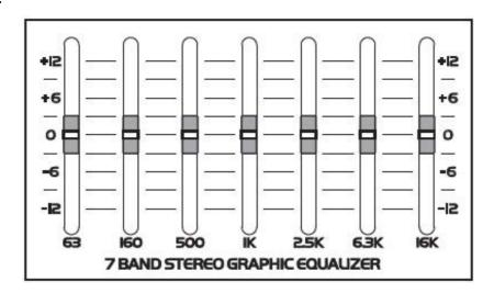
The main EQ is a stereo 7-band graphic equalizer to give overall tone shaping and can be used to help avoid feedback in live microphone setups. Each slider controls a boost or cut of up to 12dB centred at the specified frequency.
