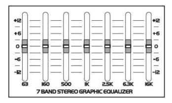
The main EQ is a stereo 7-band graphic equalizer to give overall tone shaping and can be used to help avoid feedback in live microphone setups. Each band controls a boost or cut of up to 12dB centred at the specified frequency indicated at the bottom of each slider. Running from bass to treble, these are 63Hz, 160Hz, 500Hz, 1kHz, 2.5kHz, 6.3kHz and 16kHz
